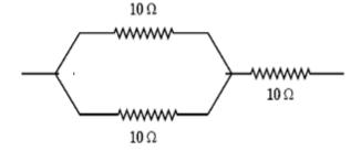
$$R = \frac{R_1 R_2}{R_1 + R_2} + R_3$$
