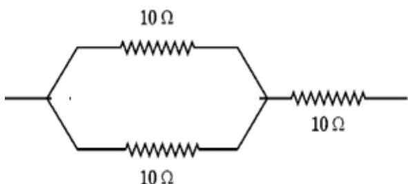
$$R = \frac{R_1 R_2}{R_1 + R_2} + R_3$$
