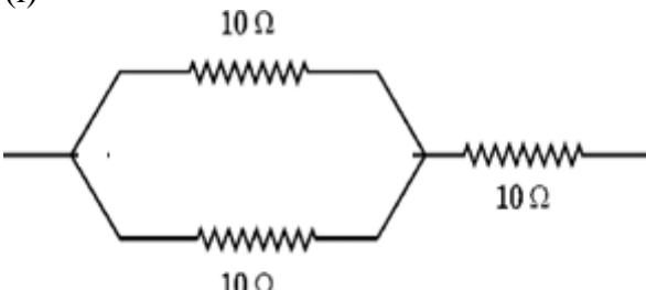
$R = \frac{R_1 R_2}{R_1 + R_2} + R_3$ $R = \left( \frac{10 \times 10}{10 + 10} + 10 \right) \Omega = 5 \Omega + 10 \Omega = 15 \Omega$
